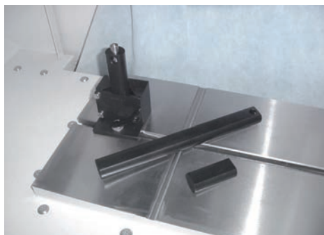
Diamond holder with exchangeable inserts (90, 150, 300 mm) for efficient circumferential and face dressing as well as calibrating.
