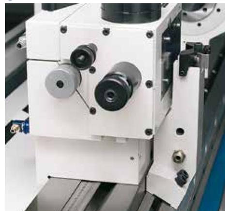
The generously dimensioned barrel, designed for the use of Morse 3 taper centres, glides in the tailstock housing. The centre pressure can be adjusted with the delicate precision required for grinding high-precision workpieces. The tailstock can be equipped with a hydraulically actuated barrel retraction for workpiece changeover. The fine adjustment enables taper corrections in the range below 1  $\mu\text{m}$  when grinding between
