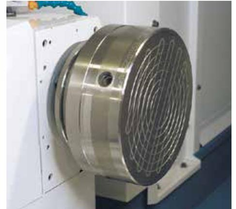
The versatile universal workhead enables both live spindle grinding and grinding between centres. The machine can also be fitted with a specially designed chuck workhead for chuck applications. The workheads are equipped with roller bearings, are low-maintenance and have an excellent roundness accuracy of under 0.0004 mm (0.000,016"), which can be optionally improved to under 0.0002 mm (0.000,008") during live spindle operations. The fine adjustment allows for taper
